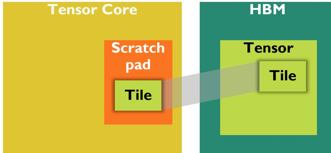
TPUs process one (fused) tensor op at a time.
